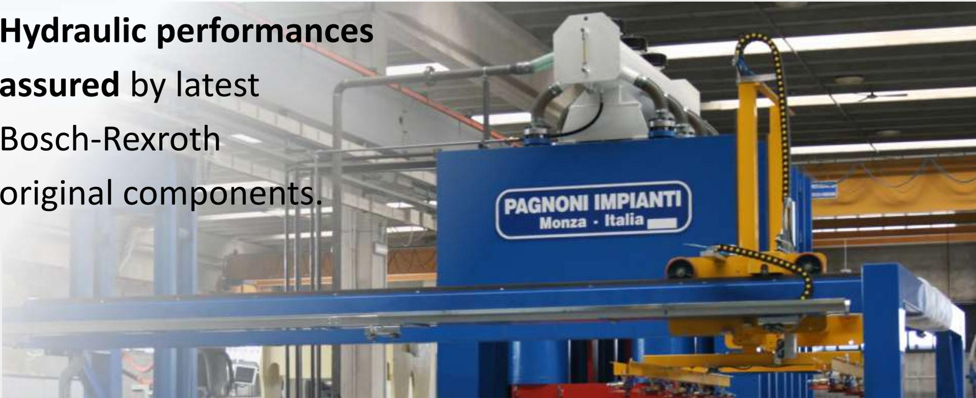
High quality **cylinders** powering Pagnoni presses to distribute an even pressure on the platen surface. Hydraulic accumulator boosting press closure speed.
